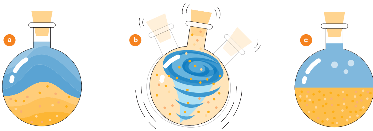
Figure 3: The behavior of sand in water: a) stagnant sand and water in a bottle; b) sand and water immediately after thorough shaking of the bottle; c) situation after several seconds as the sand settles at the bottom.
